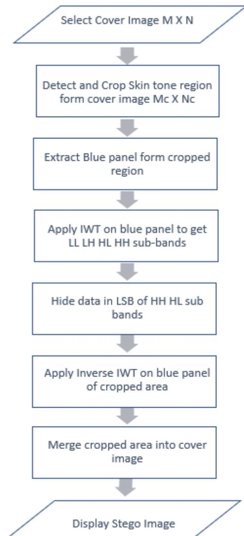
**Figure 2 Flowchart of encoding process**
